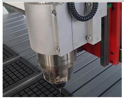
High Speed 5.5KW Water Spindle
